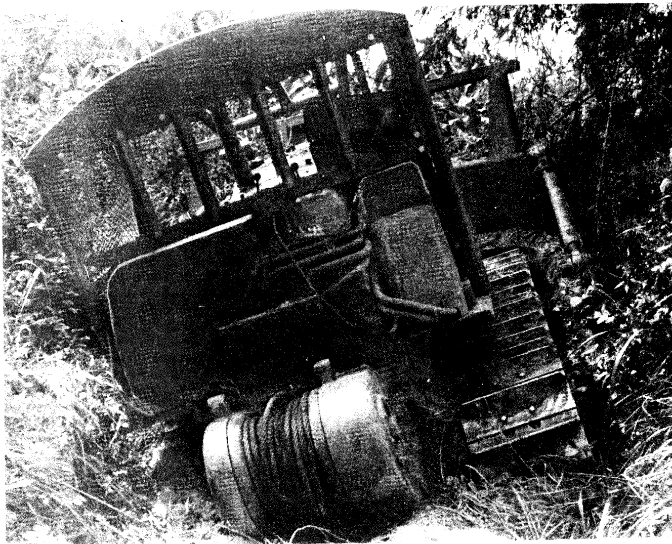
Figure C-1. Land clearing tractor that fell into an underground tunnel.
